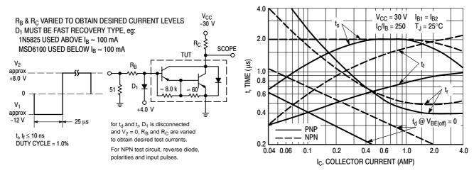
Figure 1. Switching Times Test Circuit
