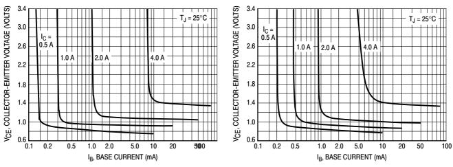
Figure 8. Collector Saturation Region
